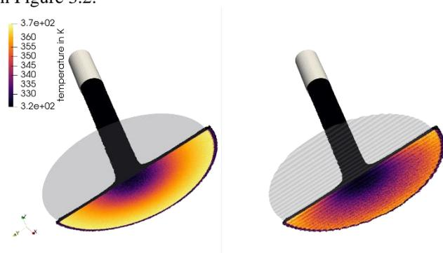
**Figure 3.2** Results of the flow simulation for a 26AWG surface for a mean inlet velocity of 5 m/s and local refinement close to the target surface (0.050 mm diameter for the coarse particles and 0.025 mm for the fine particle). In comparison to Figure 3.1 this shows a view from the bottom in order to visualize the fluid temperature at the flat (left) and 26 AWG (right) surface.
