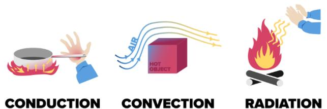
Figure 1: Examples of the three types of heat transfer.
